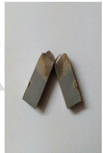
Fig 3: Specimen after Impact
